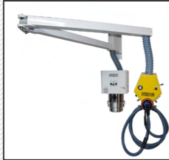
Dust Exhauster ST1-M SKU: ST1-M Supply voltage: 230V 50/60Hz Control supply: 12 Volt Suction volume: 150m 3 /h Suction vacuum : 210mbar Supply air pressure: Max 8bar Suction turbine: 1,3kW Noise: 67dBa Dimensions: 450 x 450 x 800mm
